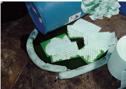
Fast containment of chemical spills.
