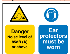
Danger Noise level of 85dB (A) or above & Ear protectors must be worn
